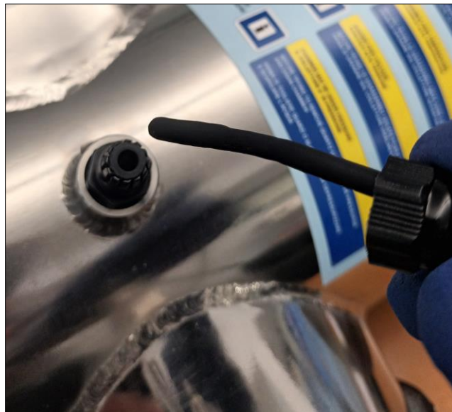
b) Insert the cable first in the cap and then in the cable gland
