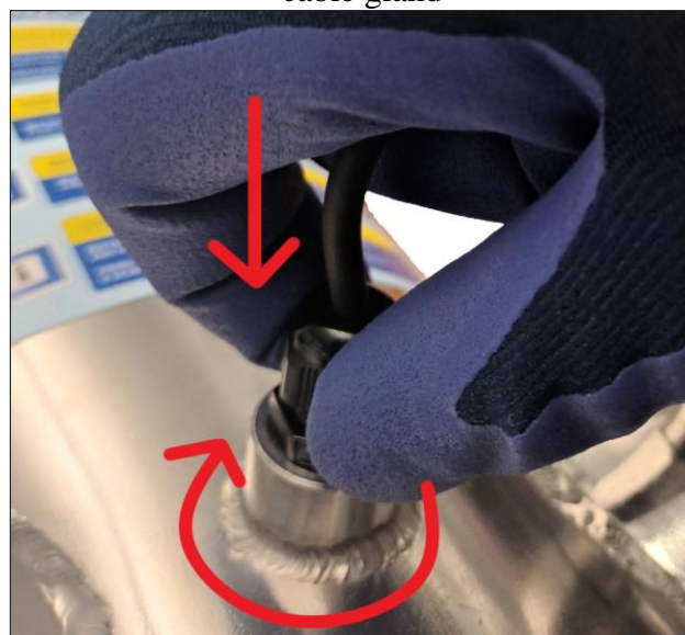
d) Screw the cap maintaining the cable pressed on the bush bottom
