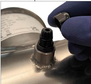
a) Remove the cable gland cap
