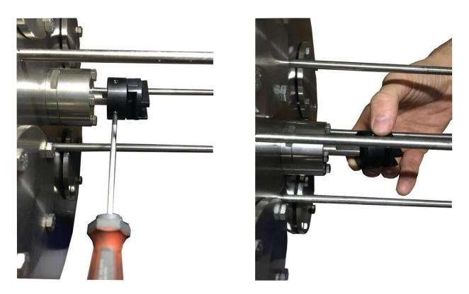
Remove seal housing by unscrewing its bolts(Use socket wrench size 8).
