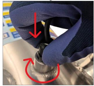
d) Screw the cap maintaining the cable pressed on the bush bottom
