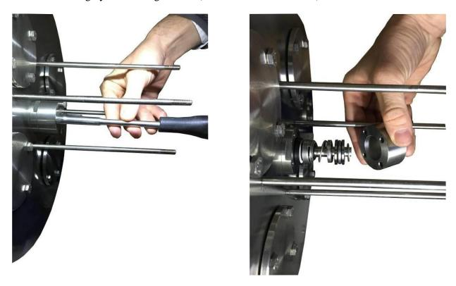
Using the screwdriver, remove the motor shaft seal and replace with the new one. Reassemble all and restart the UV system.
