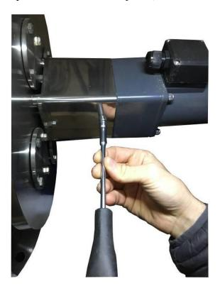
Unscrew the motor nuts and disconnect it (Use socket wrench size 10).
