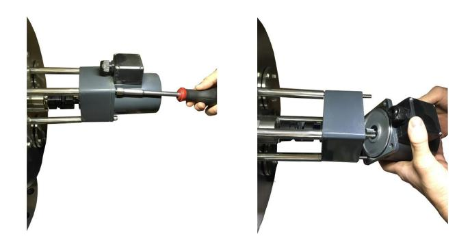
Unscrew the joint locking nut and extract it (Use Torx size 8).
