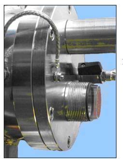
Insert the o-ring on the sleeve (point 8)
