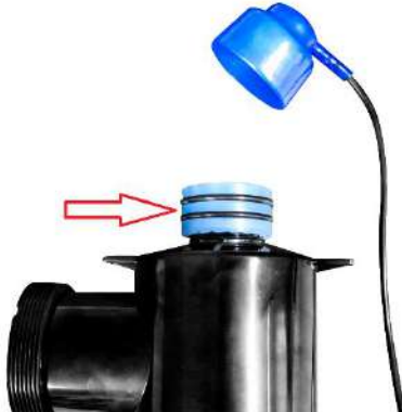
Unscrew the blue quartz sleeve locking nut anticlockwise. Both ends must be unscrewed before the quartz sleeve can be removed
