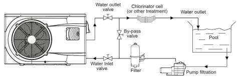
Note: The swimming pool heat pump unit is sold without any treatment or filtration equipment. The components presented in the diagram are spare parts to be supplied by the installer.
